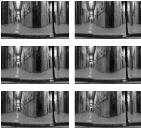
**Fig. 6. Six panoramic images, where the intermediate four are virtual images, interpolated from the first and the last image taken from the training set.**
