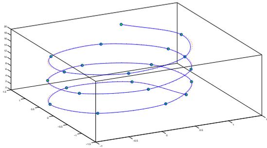
**Fig. 3** Hermite  $G^1$  interpolating spline (solid) and the  $C^2$  cubic spline interpolant (dotted) for the data, sampled from a spiral  $(\cos t, \sin t, t)$  at parameters  $t_i = 0, 1, \dots, 20$ .
