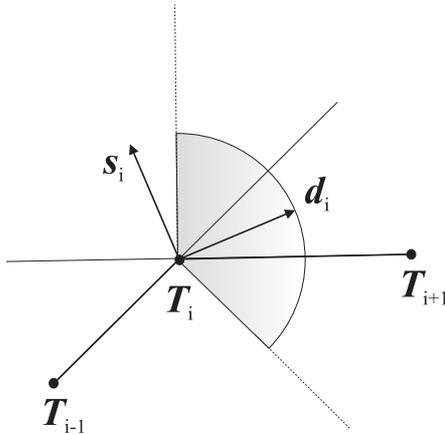
**Fig. 1** A local construction of a tangent direction  $\mathbf{d}_i$  at  $\mathbf{T}_i$ .
