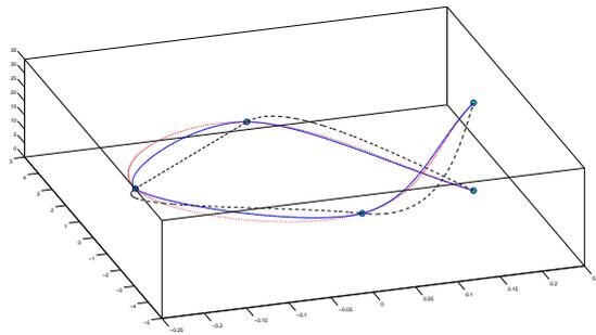
**Fig. 2** Hermite  $G^1$  interpolating spline (solid),  $C^2$  cubic spline interpolant (dotted) and Akima interpolant (dashed) of a “space” epitrochoid given by  $((R+r)\cos t - d \cos((R+r)t/r), (R+r)\sin t - d \sin((R+r)t/r), t)$  with  $R = 1.2$ ,  $r = 1$  and  $d = 2$  at the parameters  $t_i = 0, 7.85, 15.71, 23.56, 31.42$ .
